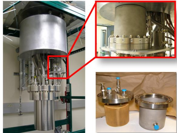
Figure 20: (Left) The PIXeY detector, fully installed, showing the position of the PIXeY two-phase heat exchanger. (Top right) A close up of the heat exchanger. (Bottom right) The heat exchanger, opened up and taken apart to show separately the inner copper pot (evaporator) and the outer steel cryostat (condenser).
